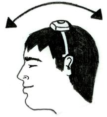
10. The LaZee Mouse™ Cursor accepts a switch input from an external switch, and uses it to reset the "home position". This provides an alternative control of the home position, in addition to the built-in switch on the top of the unit.
