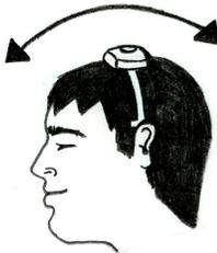
10. The LaZee Mouse™ Pro detects audio sounds via microphone, and uses them to perform click and drag functions. Spoken words, whistling, blowing, or puffing into the microphone can all be utilized to achieve the desired effect. It is completely up to the user what method to use; however, the most efficient and quietest method is to blow a puff of air, as you would if you were attempting to blow out candles.
