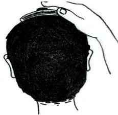
8. Imagine the head as a joystick, which controls cursor movement. Tilt the head slowly to the right (moving the ear towards the shoulder) until the computer's cursor moves to the right. Tilt the head farther to the right and the cursor will move faster. Return the head to the upright position and the cursor will stop moving
