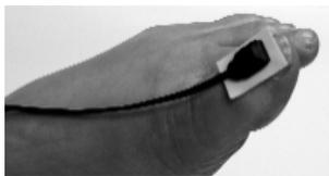
After a location has been chosen, the sensor would *ideally* be firmly attached in a level position with the cable pointing backward<sup>1</sup>. The Body sensor is very flexible in its definition of "level" meaning that it will operate effectively as long as it is within 60° of level, and can operate up to 80° with reduced performance.
