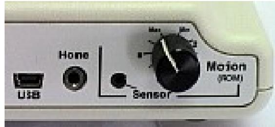
1. Initial setup should begin with a ROM setting of Max if possible. This setting provides requires the maximum amount of user movement to achieve cursor control, but is best suited for "learning" how to maneuver the sensor.
